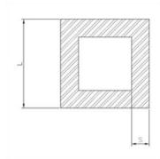
Aluminum square tubing is a type of profile made with the 1050, 1070, 3103, and 6060 alloys both in the bar and reel formats. The minimum size is 8 mm and its dimensional tolerances are +/- 0.15 mm on the side.
