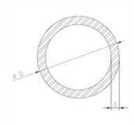
**Aluminum round tubing** is a type of profile made with the **1050, 1070, 3103, and 6060** alloys both in the bar and reel formats. The minimum size is **5 mm** and its dimensional tolerances are **+/- 0.15 mm** in diameter.
