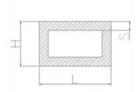
Aluminum rectangular tubing is a type of profile made with the 1050, 1070, 3103, and 6060 alloys both in the bar and reel formats. The size ranges from 12 mm to 80 mm and its dimensional tolerances are +/- 0.15 mm on the side.
